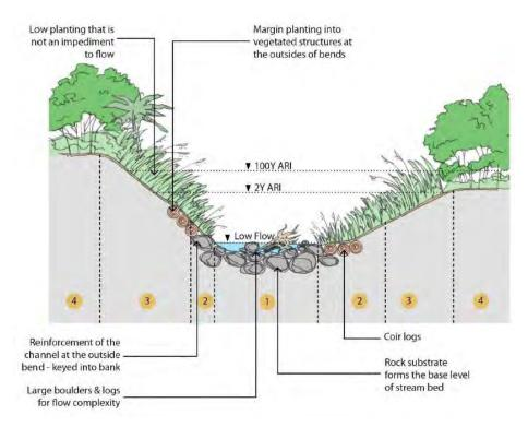
Figure 4-9: Indicative Stream Diversion Type 1 - Lowland stream cross section
