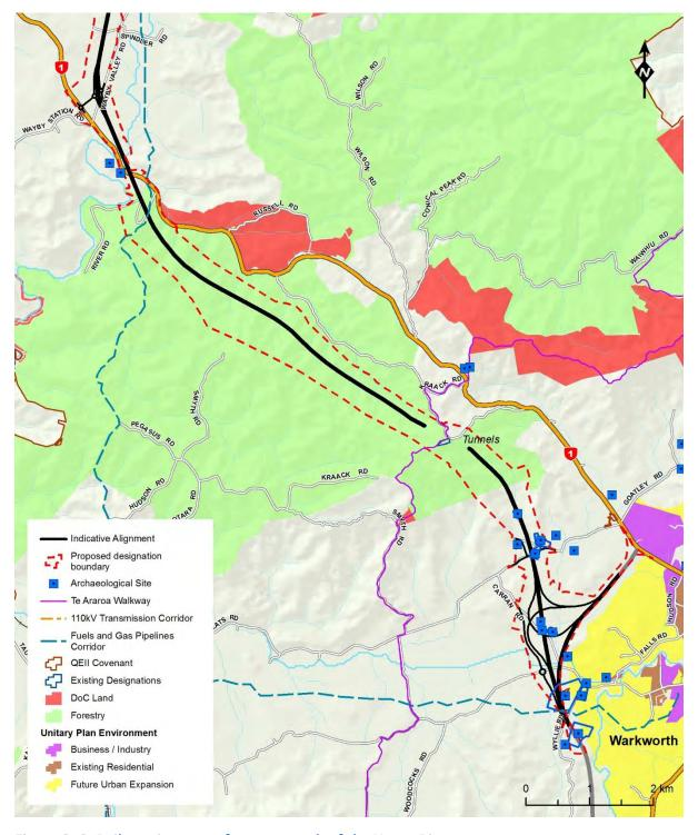
Figure 3-2: Built environment features south of the Hoteo River
